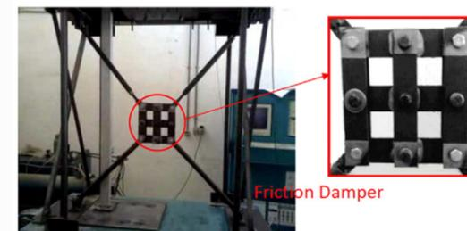
FIGURE 1.10 – Friction Damper, d'après *A modified friction damper for diagonal bracing of structures*, H.S.Monir. *Journal of Constructional Steel Research* 2013
