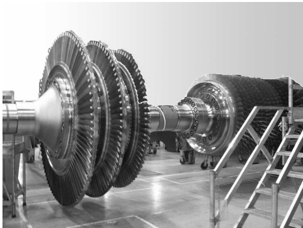
FIGURE 10 – Turbine en maintenance, Alstom
