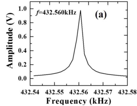
Réponse fréquentielle d'une micro poutre vibrante, d'après *Reducing intrinsic energy dissipation in diamond-on-diamond mechanical resonators toward one million quality factor, Phys. Rev. Mat., 2018*
